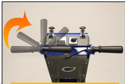
Adjustable handles and wheels makes for shot blasting as close as 3/4" to the wall
